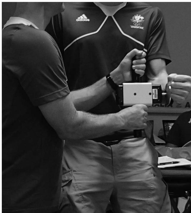
FIGURE 1—Shoulder rotation strength testing setup.
